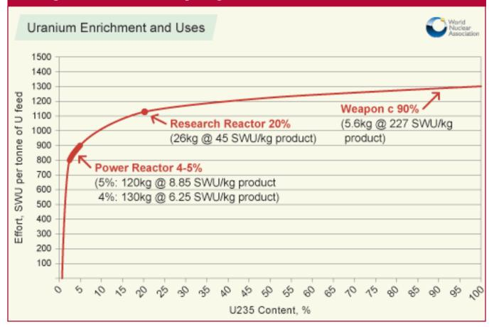
Note: In terms of the Separative Work Unit (SWU), a measure of energy used in the enrichment of U-235, the number of SWUs required per tonne of feed material (natural uranium) increases in relatively smaller increments as the desired level of enrichment rises.
